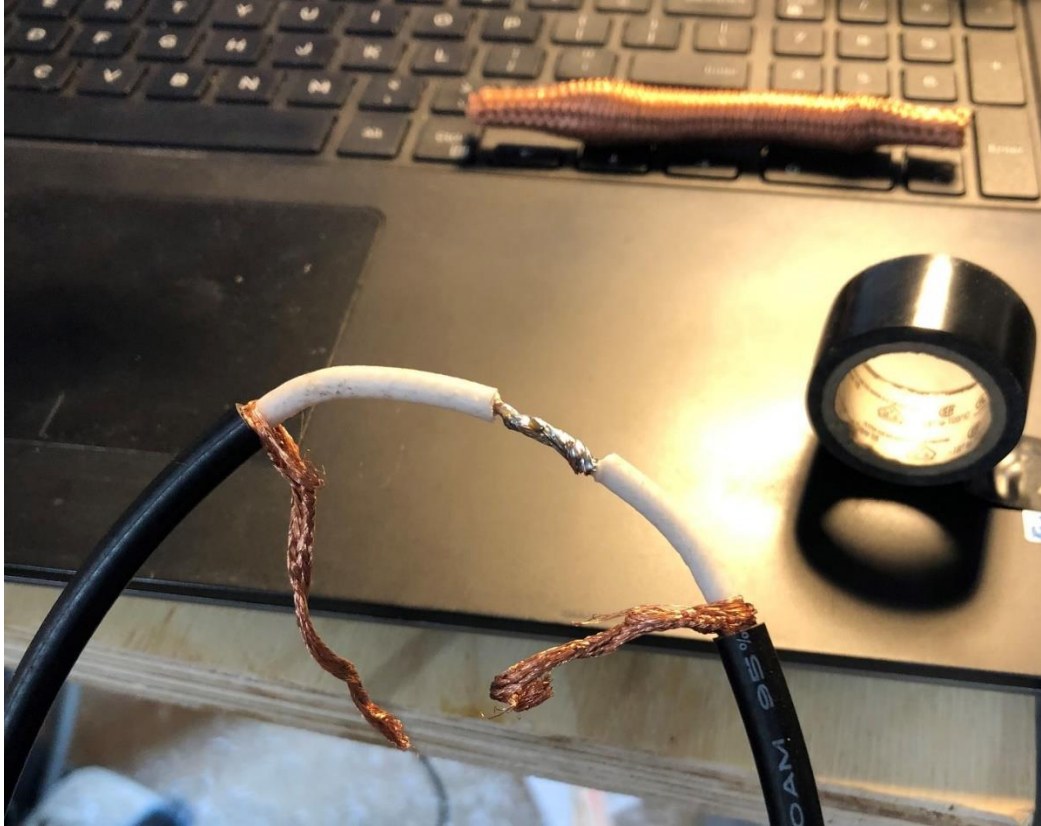
Figure 14: But surely we can do better than wire nuts. Core soldered up in telegrapher's splice
