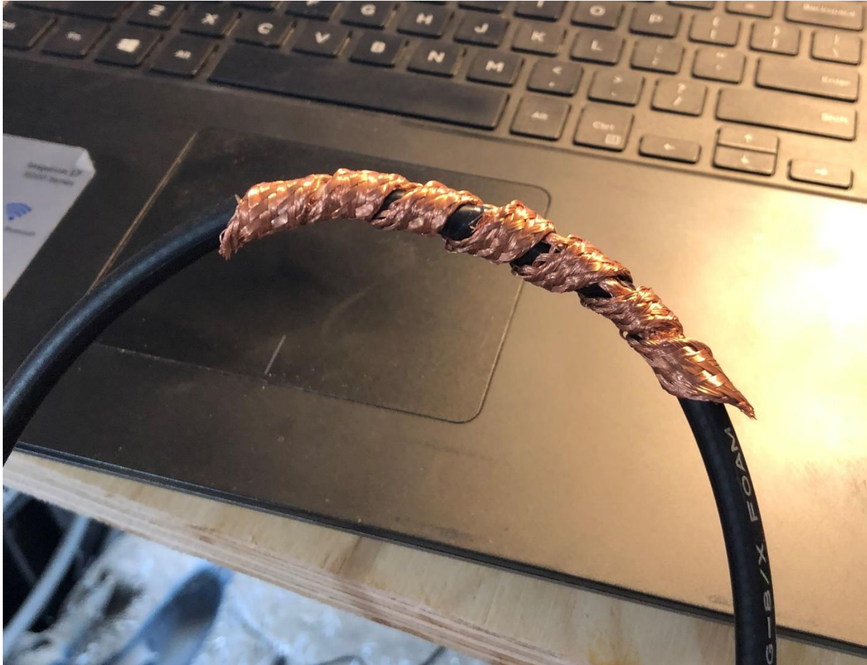
Figure 16: Taped over the telegrapher’s splice, wrapped it up in lots of copper braid. If you’ve ever had the misfortune of “makin’ it work” it might have looked like this. Then you went over it with splicing tape hoping the water would stay out.
