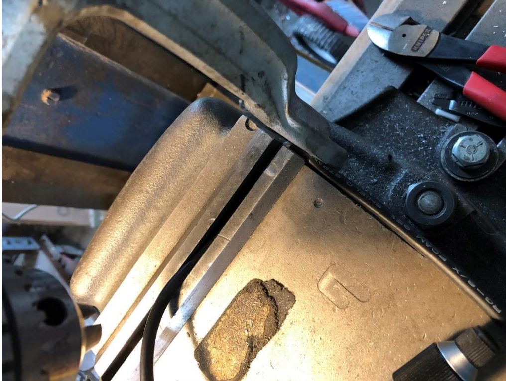
Figure 21: WAY tighter than the recommended 4.5" bend radius for RG8U. This is more like 0.01" bend radius! About like the door or trunk slam...
