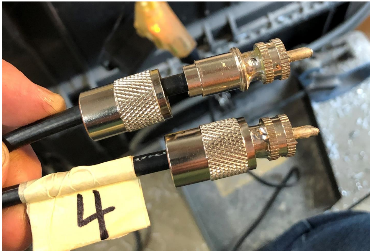
Figure 4: Yup, the ole PL259! Solder type of course. So ugly they are cute! 5/8" x 24 thread!
